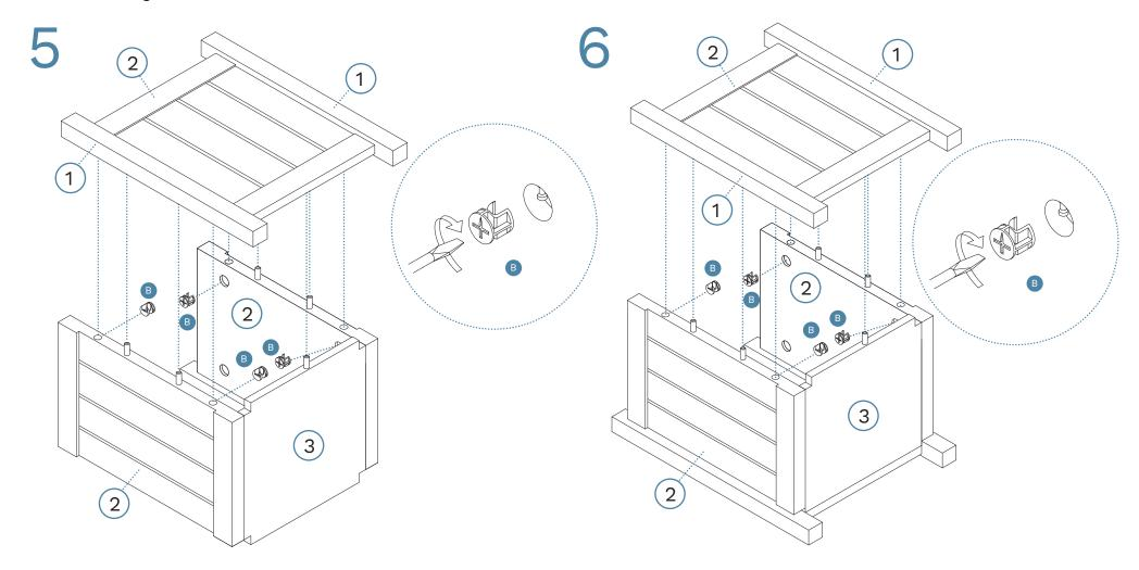
Attach panels [1] to panels [2] and [3] and secure with  $4 \times 1000$  x locking nuts (B). Tighten with a screwdriver.
